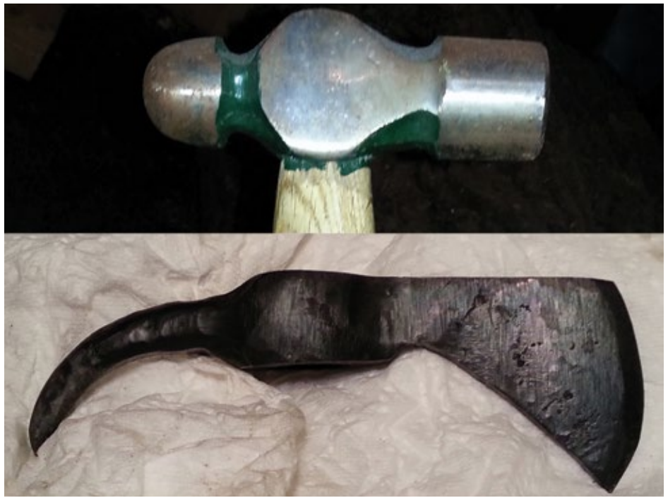
The original ball peen hammer is shown at the top while the bottom image shows the hammer after being reworked into an 18th-century style trade hatchet. Photos by author.
