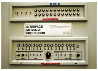
The Interface Message Processor connected UCLA to ARPANET, and relayed the first message between UCLA and Stanford.
